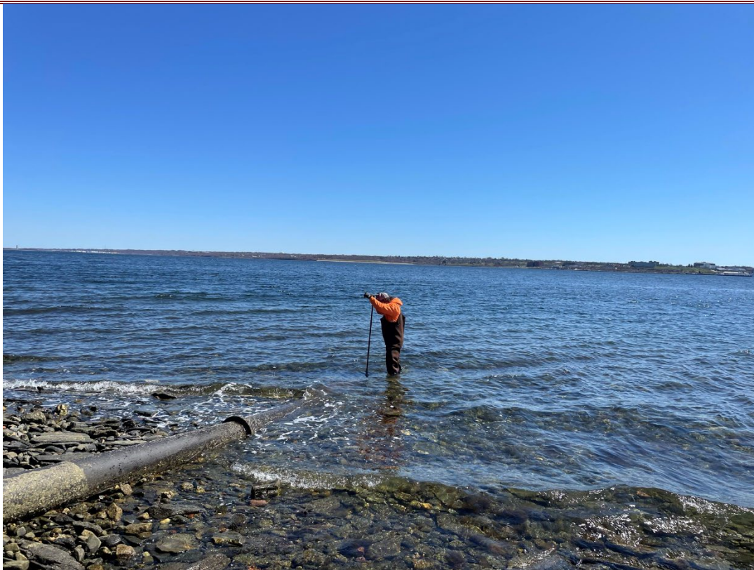
10. View of outfall sampling at submerged location (OF-14)
